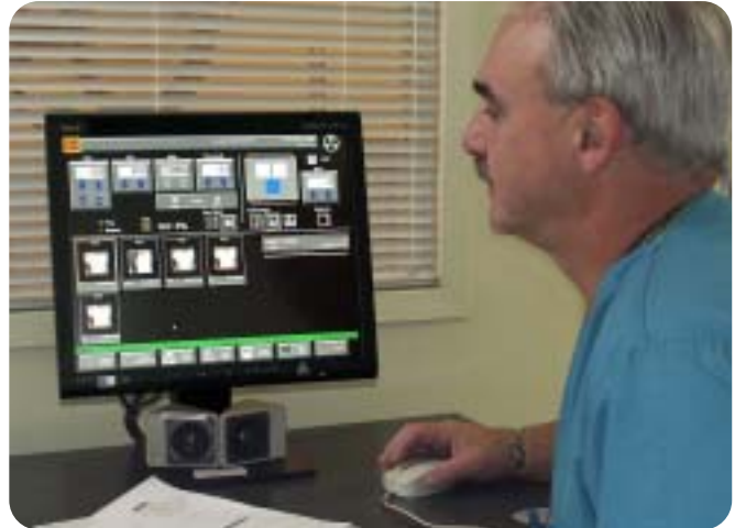
Kerry E. Lange, RT(R), prepares to take an image using the DR 7100 system. The operator interface features an easy-to-use touch screen that displays the views required and shows thumbnail images of the views that have been captured. The technologist can use either the touch screen or mouse to interact with the console.
